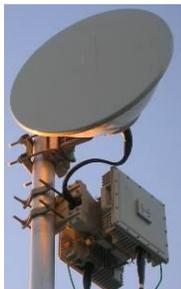
Microwave antennas have very high gains and hence are very directive, almost all the energy goes straight forward. The actual RF power applied to the antenna is typically very low. Almost always transmit power is less than 1 watt and usually around 1/10th of a watt which can be described as 100 mW or 20 dBm. **Satellite uplink (transmit) dishes that point toward the sky can have higher power and may require RF safety measures.**
